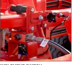
**IMPLEMENT SWITCH** The implement switch stops and starts Excelerator<sup>®</sup> is lifted in and out of work.
