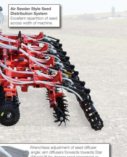
Wrenchless adjustment of seed diffuser angle: aim diffusers forwards towards Star Wheels<sup>™</sup> for deeper seed placement or rearwards towards the reel for shallower seed placement.
